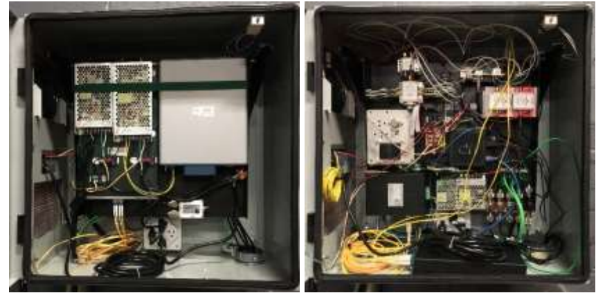
COSMOS SDR Node, SDR Tray and RF Frontend Tray
