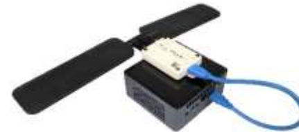
Mobile SDR Node with: B210, B205
