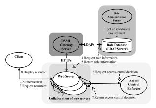
Figure 2 Operational architecture in server-pull model
