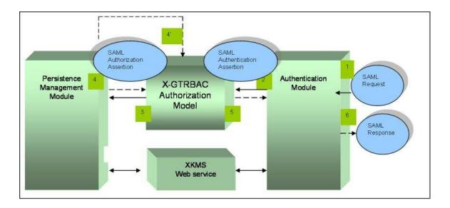
Fig. 5.2. Software architecture for the SAML profile of X-GTRBAC.
