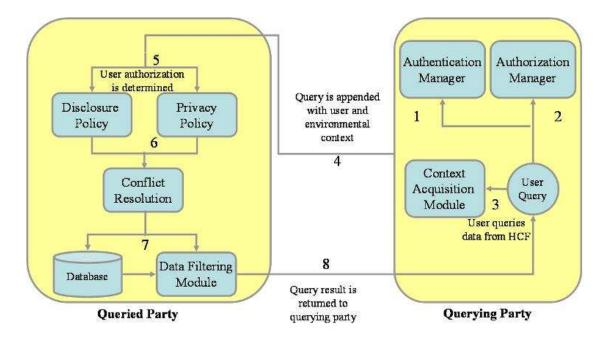
Fig. 6.1. The integrated architecture for federated healthcare database prototype.
