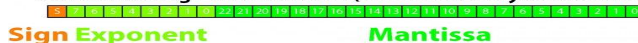
32-Bit Floating Point Notation (IEEE 754 Binary32 Standard)
